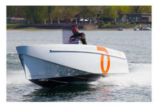
**Shell** Composite construction in high-grade structural foam with low alkali glass skin.
